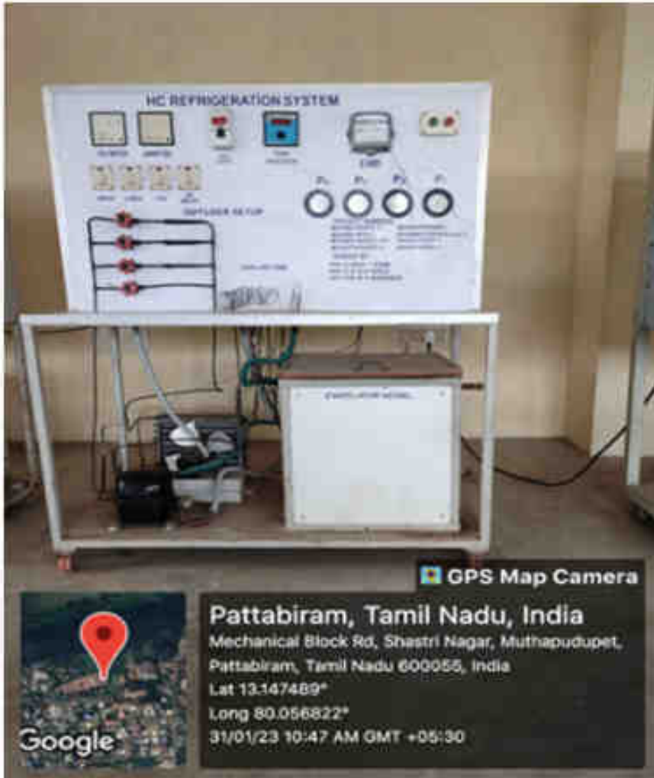
Figure 5.11. HC refrigeration system.
