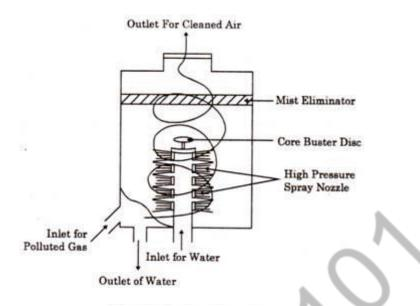
The high pressure spray nozzles generate a fine spray that intercepts the small particles in the polluted gas. The centrifugal force throws these particles towards the wall from where they are drained downwards to the bottom of the scrubber.
