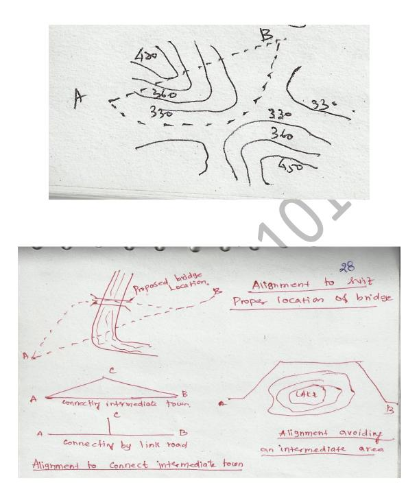
In fig.2.shows that the straight alignment between stations A and B which passes across the river band is to be deviated along the path shown in order to cross the river at a proper bridge location.
