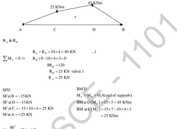
$10 \times \frac{8b^3}{12} = 27.6 \times 10^6$ b<sup>3</sup> =  $\frac{27.6 \times 10^6 \times 12}{10 \times 8} = 4140000$ b = 160.57 d = 2 b = 321.14 mm
