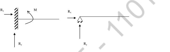
Resistance to the moment m = 0NDisplacement at (x & y axis)R $u_x = 0$ u $u_y = 0$ u
