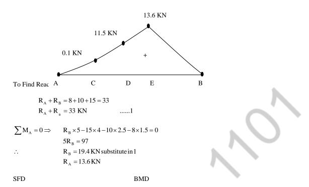
SF at B = -13.6 KN SSB at supports  $M_A = M_B = 0$ SF at E = -13.6 + 15 = 1.4 KN SF at D = -13.6 + 15 + 10 = 11.4 KN $M_{\rm E} = 13.6 \times 1 = 13.6 \, \rm KNm$ SF at C = -13.6 + 15 + 10 + 8 = 19.4 KN M<sub>D</sub> =  $13.6 \times 2.5 - 15 \times 1.5 = 11.5$  KNm SF at A = 19.4 KN
