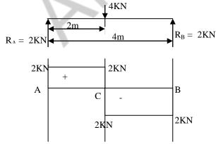
$$R_{A} + R_{B} = 4KN$$
