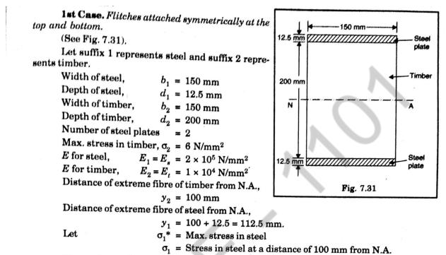
Now we know that strain at the common surface is same. The strain at a common distance of 100 mm from N.A. is steel and wood would be same. Hence using equation (7.11), we get
