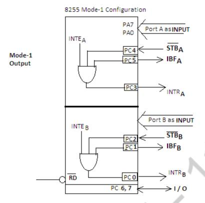
**STB** (**Strobe Input**): This signal (active low) is generated by a peripheral device that it has transmitted a byte of data. The 8255, in response to, generates IBF and INTR.
