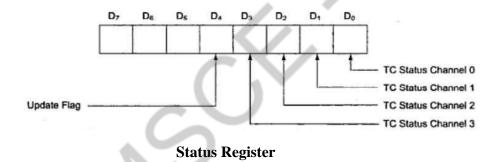
These bits remain set till either the status is read by the CPU or the 8257 is reset.
