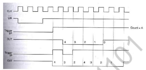
WR, GATE and OUT Waveforms in Mode 1
