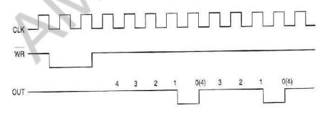
Waveforms at pin WR and OUT in Mode 2  $\,$
