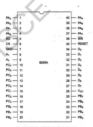
Fig. 5.17(b) 8255A Pin Configuration
