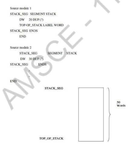
Fig.1.10 Formation of a stack from two segments
