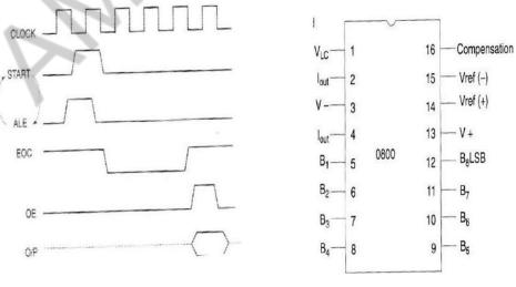
Timing Diagram of ADC 0808/0809
