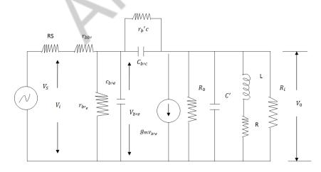
**16.**Determine the bandwidth of two stage synchronous tuned amplifier. Assume the bandwidth of individual stage is 310 KHz[**APRIL/MAY 2014**]
