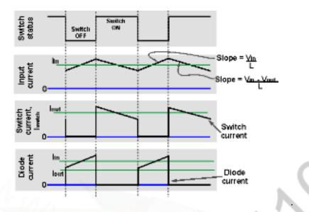
It can be seen from the waveform diagrams that the input current to the boost converter is higher than the output current. Assuming a perfectly efficient, i.e. lossless, boost converter, the power out must equal the power in, i.e.  $Vin \cdot Iin = Vout \cdot Iout$ . From this it can be seen if the output voltage is higher than the input voltage, then the input current must be higher than the output current.
