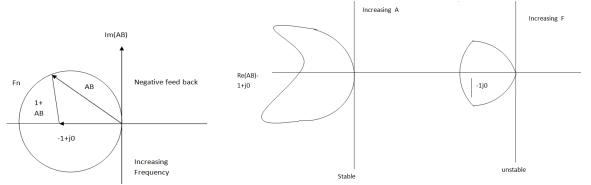
The criterion of Nyquist is that, the amplifier is unstable if this curve encloses the point -1 + jo, and the amplifier is stable if the curve does not enclose this point. Locus of  $11 + A\beta I = 1$
