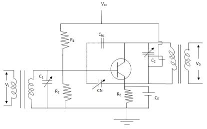
In this circuit, the neutralization capacitor is connected from the lower end of the base coil off the next stage to the base of the transistor.
