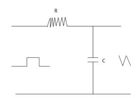
It consists of series resistor and a shunt capacitor. This circuit passes low frequencies of the input and alternates high frequencies because the reactance of the capacitor C decreases with increasing freq. At the very high frequencies, the capacitor acts as a virtual short circuit and the output falls to zero. Hence this circuit is called low pass filter.
