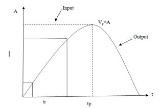
If the rise time  $t_r$ , is equal to  $0.35t_p$ , then the output is reproduction of the input.
