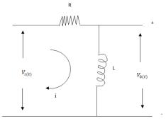
It consists of a series resistor (R) and shunt inductor (L).  $X_L = 2\pi f L$  at f = 0, the realtance becomes zero, and inductor acts as a short circuit and the o/p falls to zero. Since the inductor acts as a short circuit, for a certain low freq range, the circuit doesnot pass low freq of the input.
