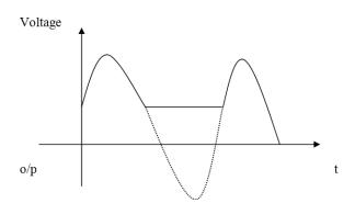
Here the entire signal below  $+V_R$  is clipped off. 4. <u>Combination Clipper</u>
