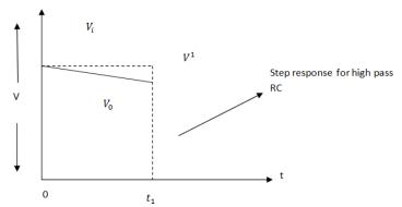
The response  $V_o$  which exhibits a tilt when a step  $V_i$  is applied to a high pass RC circuit. Since the capacitor is initially uncharged, the o/p at t=0, will be V.  $V_o = e^{-t/RC}$ .
