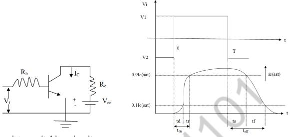
Transistor switching circuit.
