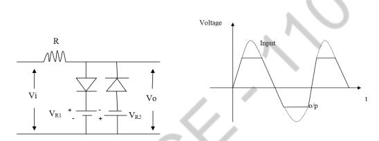
When the input signal voltage  $V_i \ge +V_{R1}$  diode  $D_1$  conducts and acts as a closed switch, while diode  $D_2$  is reverse biased and  $D_2$  acts as open switch. Hence the output voltage cannot exceed the voltage level of  $+V_{R1}$  during the positive half cycle.
