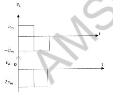
During the first quarter of positive cycle of the input voltage  $V_i$ , the capacitor gets charged through forward biased diode up to maximum value  $V_m$ .
