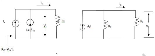
Applying KCL to the input node,  $I_s - I_i - I_f + I_f = o$   $I_s = I_i + I_f$   $= I_i + \beta I_o$ O/p Current  $I_o$  is given as,  $I_o = \frac{A_i I; R_o}{R_o + R_L}$   $I_o = A_I I;$ Substituting the value of  $I_o$ ,  $I_s = I_i + \beta A_i I;$   $I_s = I(1 + \beta A_I)$   $R_{if} = \frac{V_i}{I_s} = \frac{V_i}{I_i(1 + \beta)_I}$  $R_{if} = \frac{R_i}{(1 + \beta)_I}$
