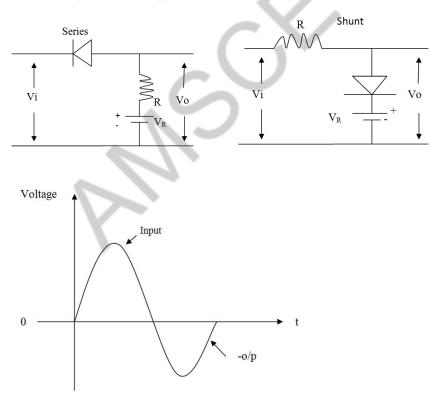
Here the entire signal above  $-V_R$  is clipped off. (iii) <u>Biased negative clipper</u>
