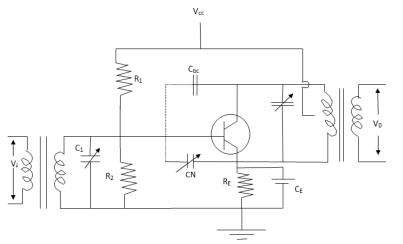
In this circuit, a small value of variable capacitance  $C_N$  is connected from the bottom of coil, point B to the base. Therefore the internal capacitance  $C_{bc}$ , feeds a signal from the top end of the coil, point A, to the transistor base and  $C_N$  feeds a signal of equal magnitude but opposite polarity from the bottom of the coil, point B to the base. The neutralizing capacitor  $C_N$  can be adjusted correctly to completely nultify the signal fed through the  $C_{bc}$ .
