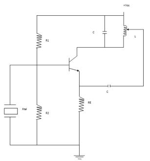
The Miller crystal controlled oscillator is shown. The crystal has two resonant frequencies. In between Ws & Wp, the reactance of the XTAL becomes inductive and hence can be used as inductor. One of the inductor in Harley OSC can be replaced by the crystal which acts as an inductor when freq is greater than Ws. The inter electrode capacitance is used as a capacitor to generate the oscillations. <u>Pierce Crystal Oscillator</u>
