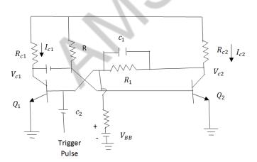
Monostable multivibrator has one stable state and on quasi-stable state. It is also known as one shot multivibrator or univibrator. It remains into its quasi-stable state for a time determined by discharging an RC circuit and the circuit returns to its original stable state automatically.
