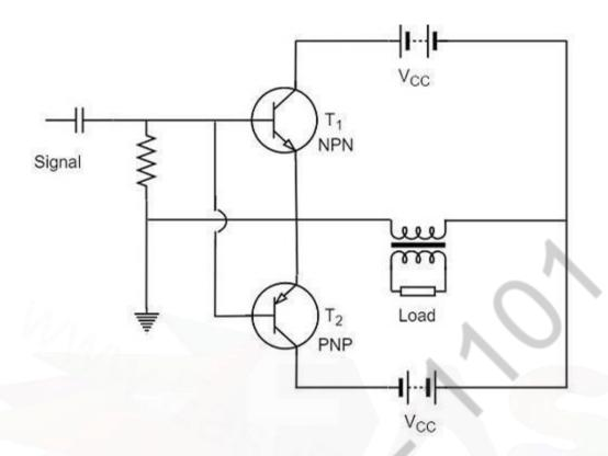
The above circuit employs a NPN transistor and a PNP transistor connected in push pull configuration. When the input signal is applied, during the positive half cycle of the input signal, the NPN transistor conducts and the PNP transistor cuts off. During the negative half cycle, the NPN transistor cuts off and the PNP transistor conducts.
