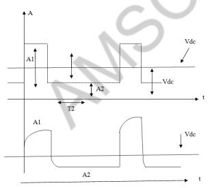
When the time constant of the circuit is very small, the output is almost similar to the input.
