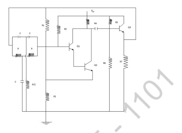
This circuit consists of Darlington Pair ( $Q_1$  and  $Q_2$ ) and it is followed by emitter follower ( $Q_3$ ). The Twin-T network is used as the feedback circuit, which is used as a notch filter. The Darlington pair circuit proves 180° phase shift and the feedback network also introduces 180° phase shift. The total phase shift around the circuit is 360° or 0°. The twin-T network oscillator yields better freq stability.
