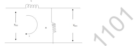
It consists of a series inductor and a shunt resistor. The circuit passes low frequencies of the input and alternates high frequencies because the reactance of the inductor L is directly proportional to the frequency. At very high frequencies, the inductor acts as a virtual open circuit and the output falls to zero. Hence this circuit is called low pass filter.
