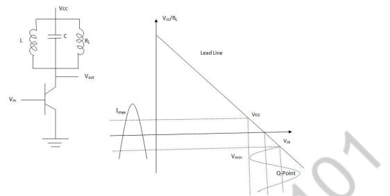
The large signal tuned amplifiers amplify high power signals of the radio freq range using class-c operation rather than class-A.
