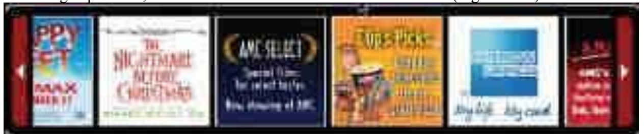
Figure 7-13. If AMC animates its carousel backward from the accepted standard, clicking the right arrow should scroll the content from the right (not the left)
