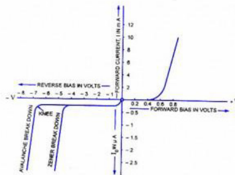
Fig 1.18: Diode characteristics with breakdown
